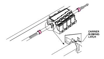
Figure 5-11. Carrier Bushing Removal.
